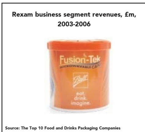
"In October 2006, Ball launched Fusion-Tek, a new microwavable steel can. The can, which uses recycled steel, has a plastic bottom. A normal steel food can does not heat in the microwave because microwave energy cannot pass through steel, but Fusion-Tek's plastic end allows microwave energy to pass through the product inside the can, heating it quickly and evenly in 2-3 minutes..."
